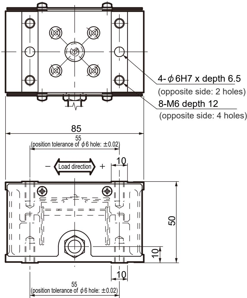
Note: In the factory setting mode, the amplifier output value will increase when the load is applied in the "+" direction of the double arrow sign.
