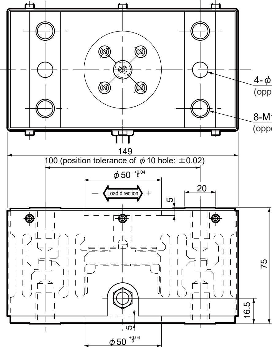
Note: In the factory setting mode, the amplifier output value will increase when the load is applied in the "+" direction of the double arrow sign.
